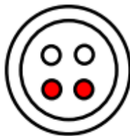
Figure 1: Parallel construction of the Duplex (4-wire) Thermocouple Cable. This is the standard configuration made at Idaho Labs.
