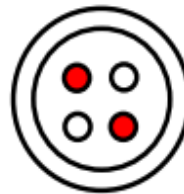
Figure 2: Diagonal Construction of Duplex Cable. The red circles denote negative wires. This configuration is available upon request. Known as alternating or "DIAG".
